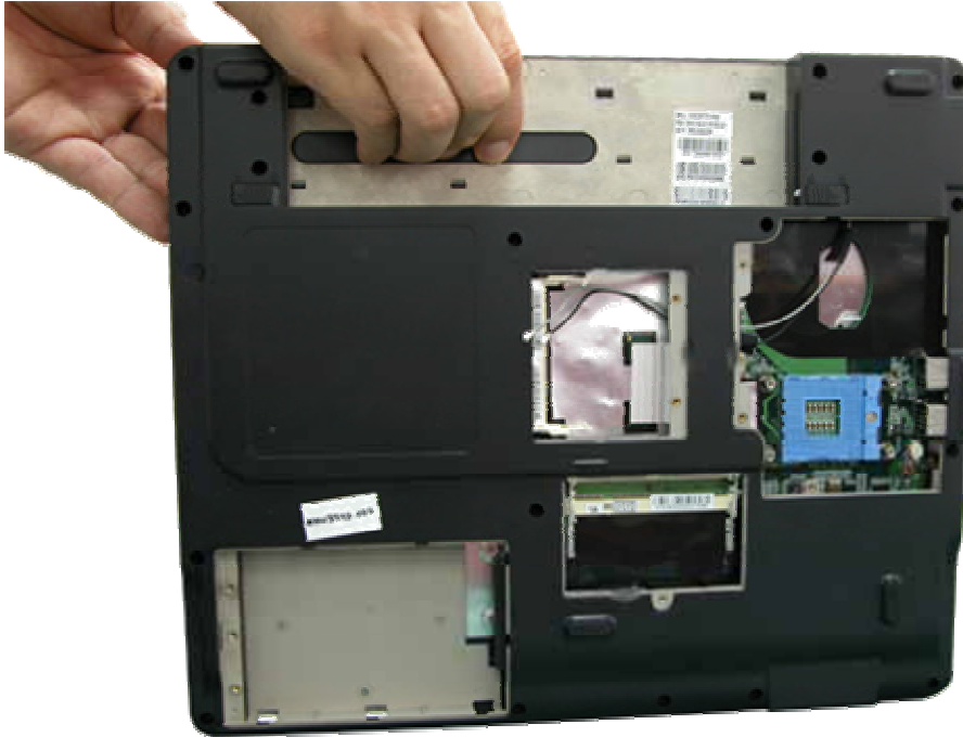
Fig. 14 Releasing the keyboard cover
